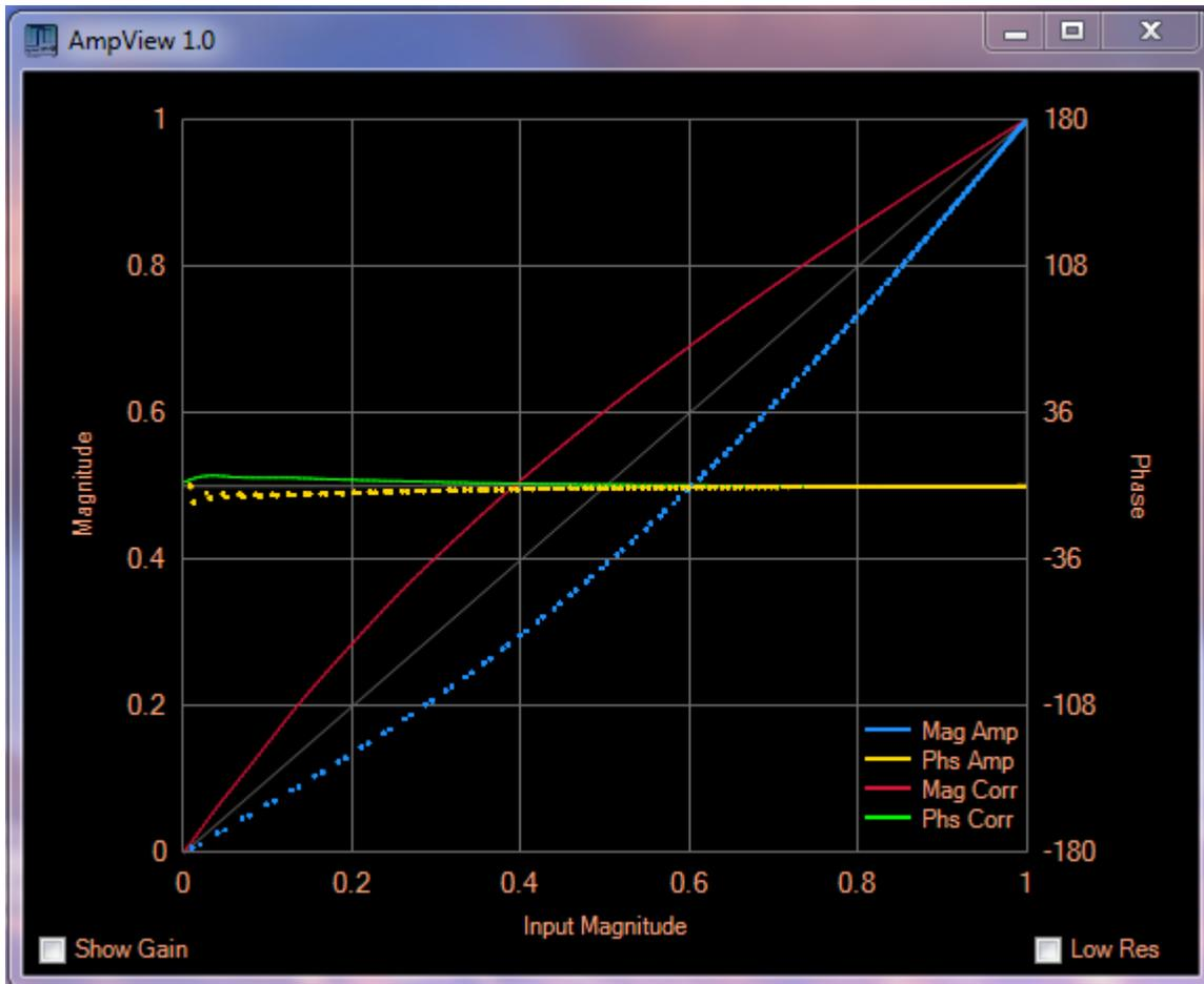
The blue dots show the output magnitude versus input magnitude of the uncorrected amplifier. Similarly, the yellow dots show the uncorrected phase characteristic versus input magnitude for the amplifier. Note that these are discrete dots at the points of the samples collected to perform the PureSignal calibration. The red and green lines then show the calculated magnitude and phase corrections that are being applied to outgoing transmit samples.
