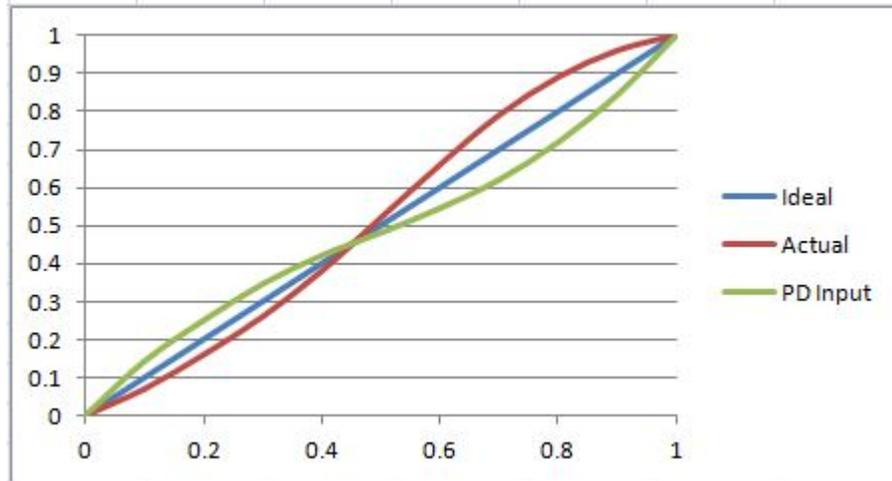
In addition to the amplitude distortion shown in the above figures, there is also a phase distortion (amplifier phase shift varies as a function of signal amplitude) that must be corrected to achieve significant reductions in IMD.
