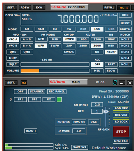
FIGURE 1: Typical SDR UNO settings to make the necessary recordings.
