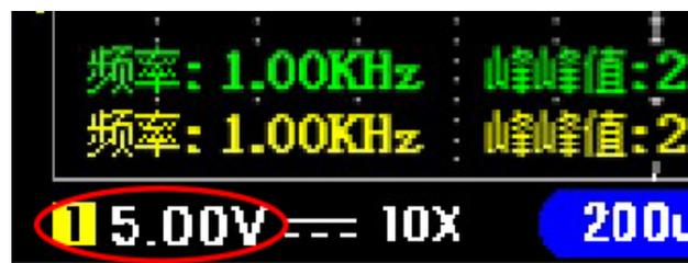
The scope's vertical sensitivity range is 10mV / div ~ 10V / div (1X probe). In the oscilloscope button panel, the keys for adjusting the vertical sensitivity are 'mV' and 'V' button. Pressing the 'mV' button decreases the vertical sensitivity, which is used to measure signals with smaller voltage amplitude. Press the 'V' button to increase the vertical sensitivity for measuring signals with larger voltage amplitudes.
