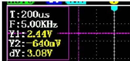
Press the left and right arrow keys directly to move the horizontal cursor 1. After pressing the Shift key, press the horizontal arrow key again to move the horizontal cursor 2. The same goes for vertical cursors.
