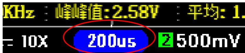
The oscilloscope time base range is 5ns ~ 10s. The buttons for adjusting the time base in the oscilloscope button panel are 'ns' and 's' button. When observing high-frequency signals, you should press the 'ns' button to decrease the time base. When observing low-frequency signals, you should press the 's' button to increase the time base. The time base in the figure is 200us/div.
