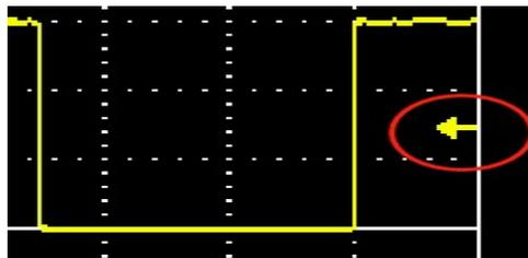
The arrow circled above is the trigger level position, and when the edge of the square wave in the above figure passes upwards through the position of this arrow, a trigger is formed (the waveform only forms a trigger when it crosses the trigger level up or down).
