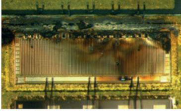
Figure 3: Example of a thermal device failure as a result of high dissipation
