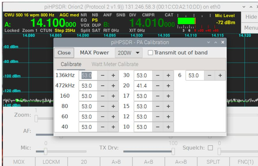
**Fig. 8.2:** The PA menu, PA calibration screen
