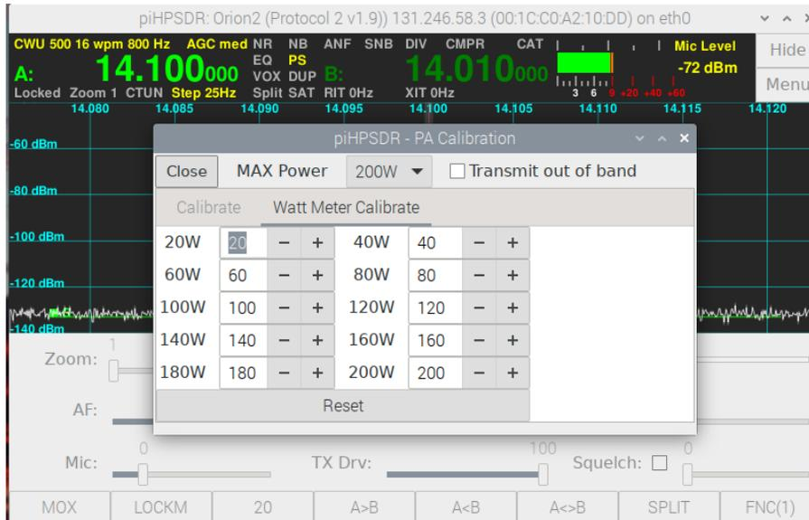
**Fig. 8.3:** The PA menu, Watt meter calibration
