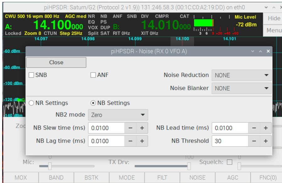
**Fig. 7.5:** The **Noise** menu (with NB settings).
