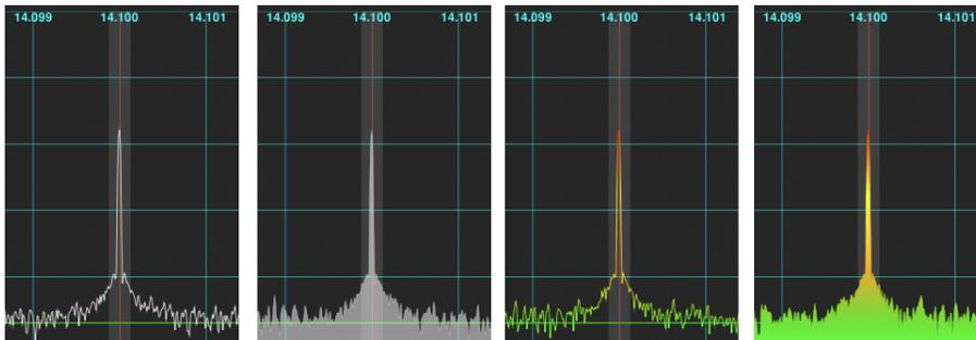
**Fig. 3.2:** Display options for the spectrum scope.
