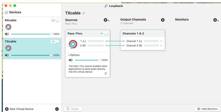
**Fig. F.9:** Setting up „loopback” on MacOS, TXcable
