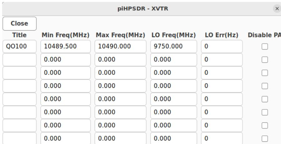
Fig. 5.9: XVTR setup for QO-100 operation.
