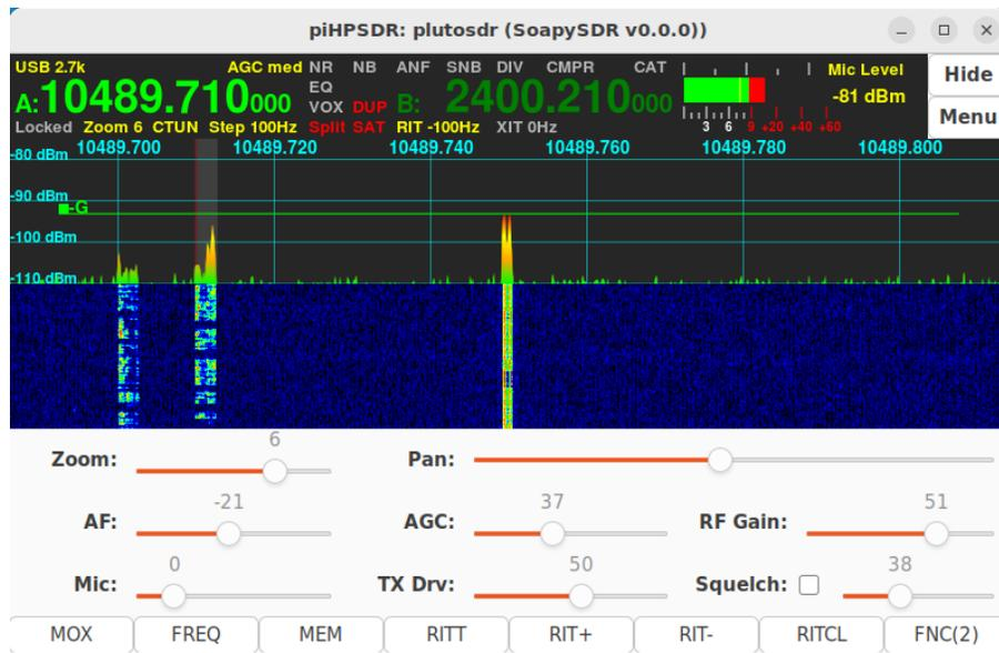
Fig. 5.11: Working QO100 with piHPSDR and the Pluto.
