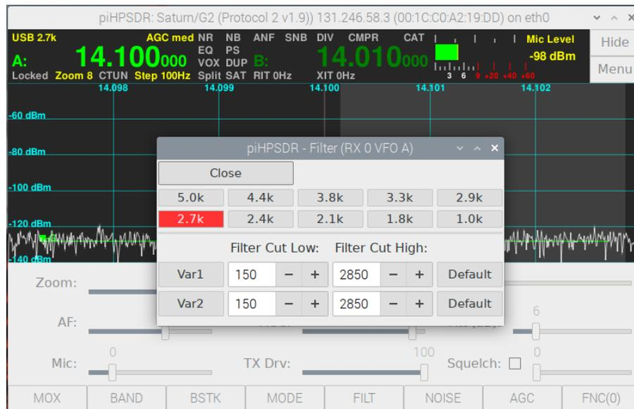
**Fig. 7.2:** The [Filter](#) menu (single side band modes).
