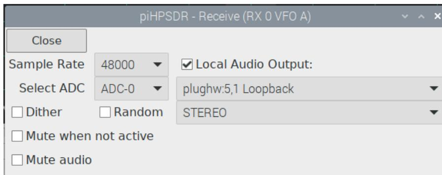
**Fig. F.1:** RX menu settings for using loopback with ALSA.
