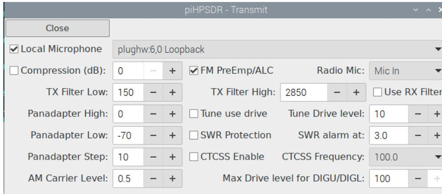
**Fig. F.2:** TX menu settings for using loopback with ALSA.
